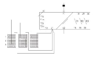
The Y1 line controls the maximum/minimum level of the D1 tank. The same for line Y2 and tank D2. Line Y3 controls a single level in tank D3. For this application it is very important to install an independent electrode as a reference (common) from each tankupto terminal Z1.
