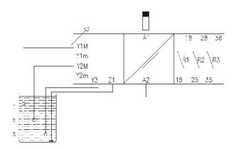
Relays R1, R2 and R3 are activated when the liquid level comes into contact with electrodes Y1m, Y2m and Y3 respectively. The relays are deactivated when the liquid drops below each of the electrodes.
