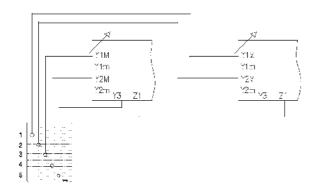
In this application, the reference electrode (common) can be the same to be connected to the Z1 terminals when the SNZA controls the same tank.
