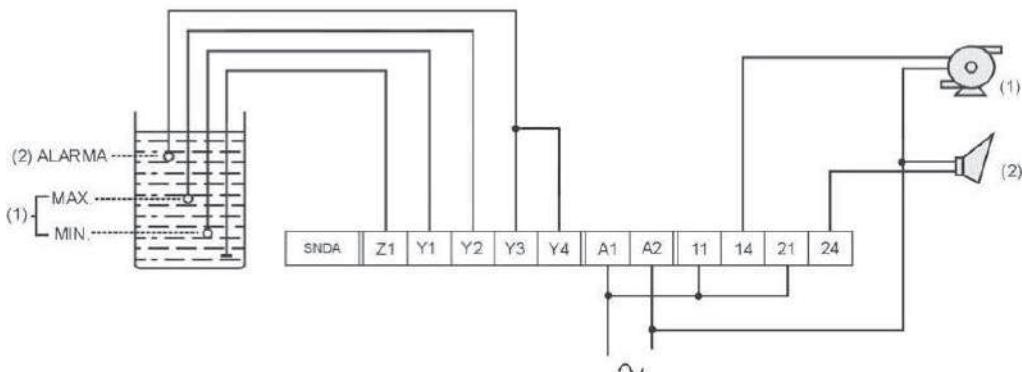
**Emptying control of two separate tanks**
