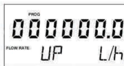
In a CH420R, if during the programming sequence we receive a HART command that must be attended, the local programming will not be valid and all the data previously programmed will be lost. The screen will return to the normal working model and the word PROG will light on the screen, indicating this event. To remove the word PROG from the display, press any of the two PROG push buttons.
