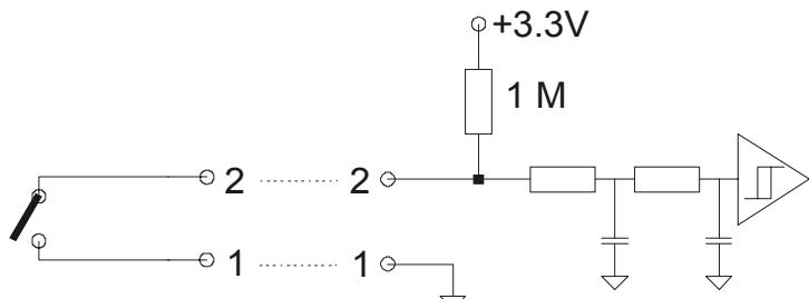
Due to the presence of a filter to avoid the effects of contact bounce, the maximum pulse frequency for the COVol input is 300 Hz.
