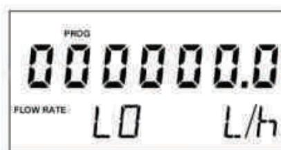
In the first screen we program the flow rate equivalent to 4 mA (lower range). The measuring units will be the ones chosen in the previous screen. The push buttons have the same function as the pulses per litre programming.
